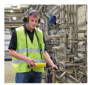
integrated suction pump available which allows you to detect even the smallest concentrations of trace gas.
