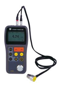
Time Group ultrasonic thickness gauges measure the thickness of ultrasonic wave wellconductive materials with parallel top and bottom surfaces. It measures the thickness of both metal (steel, aluminum, titanium, etc.) and nonmetal (plastics, ceramics, glass, etc.) parts. They are commonly used to measure (remaining) wall thickness of pipes and pressure vessels.
